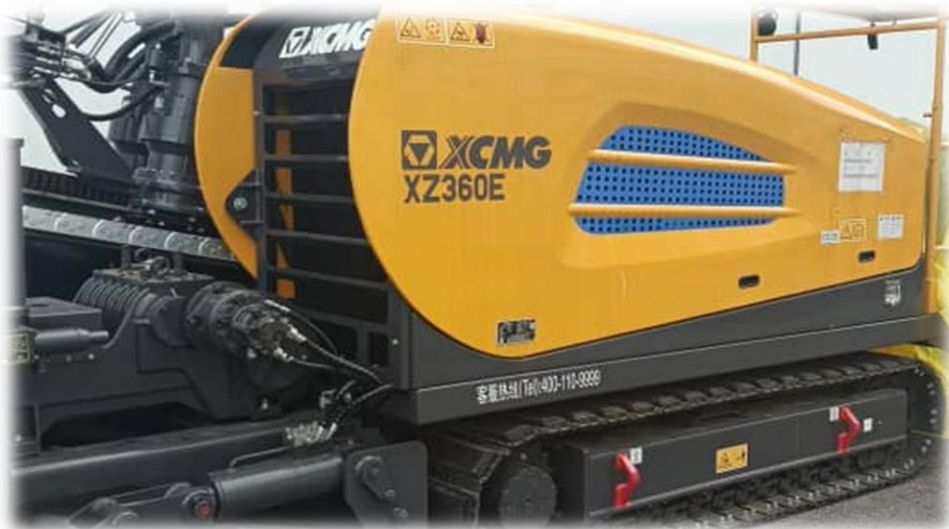
7 th HDD MACHINE 36 TONNE
