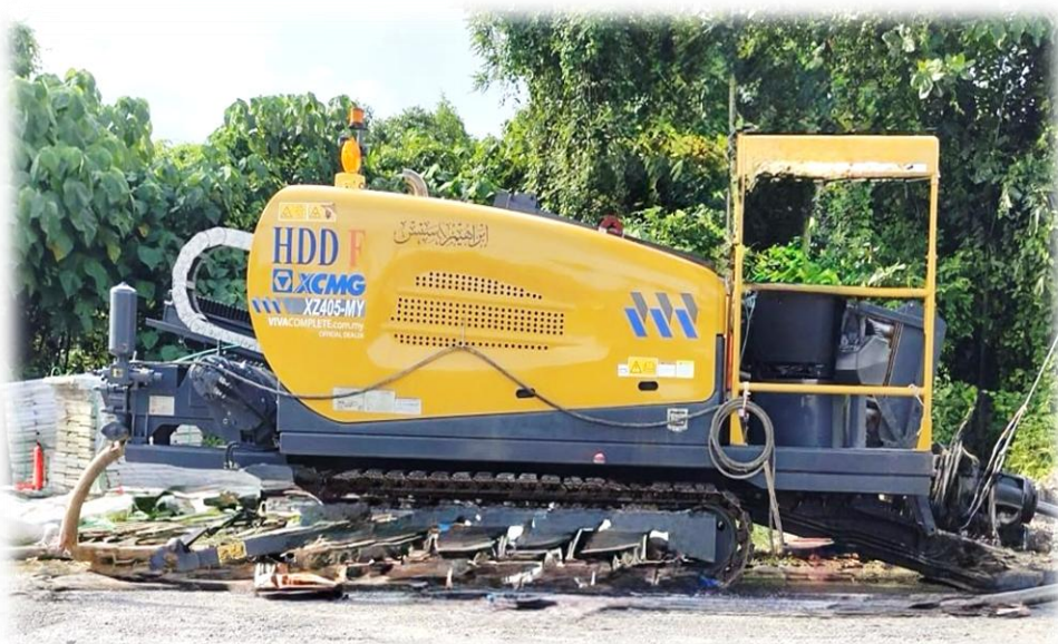
9 th HDD MACHINE 40 TONNE
