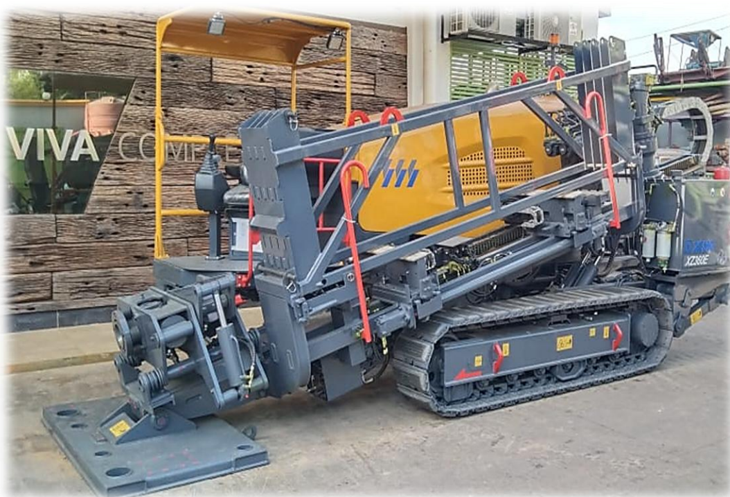
4 th HDD MACHINE 36 TONNE
