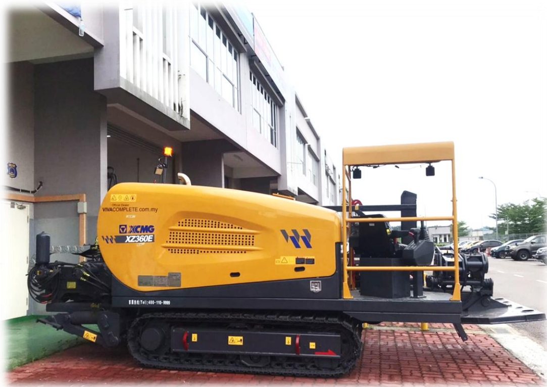
1 st HDD MACHINE 36 TONNE
