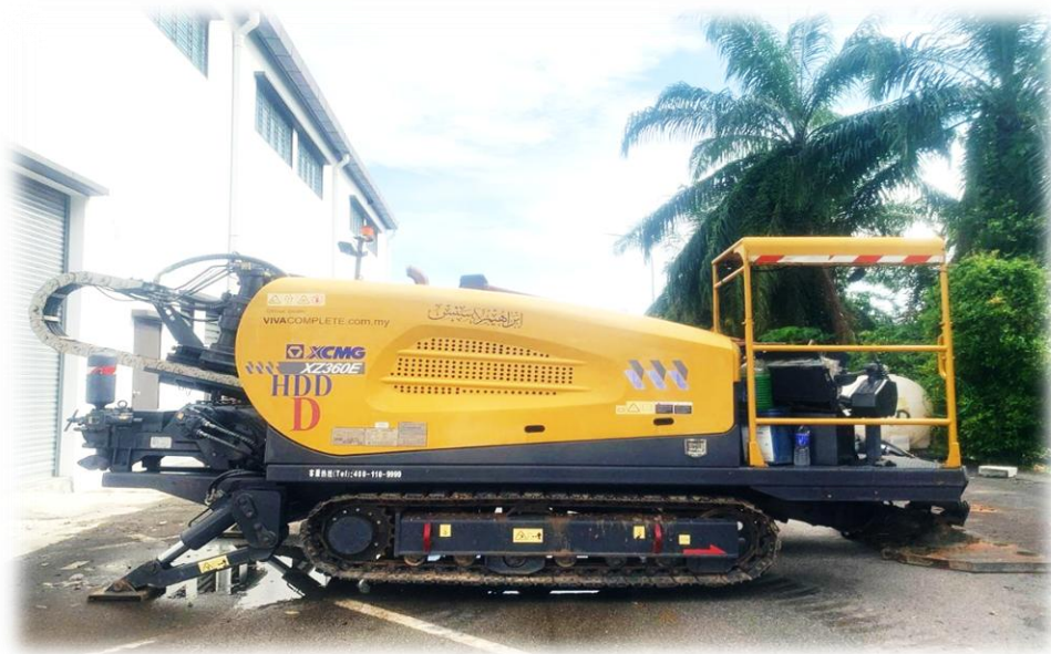
8 th HDD MACHINE 36 TONNE
