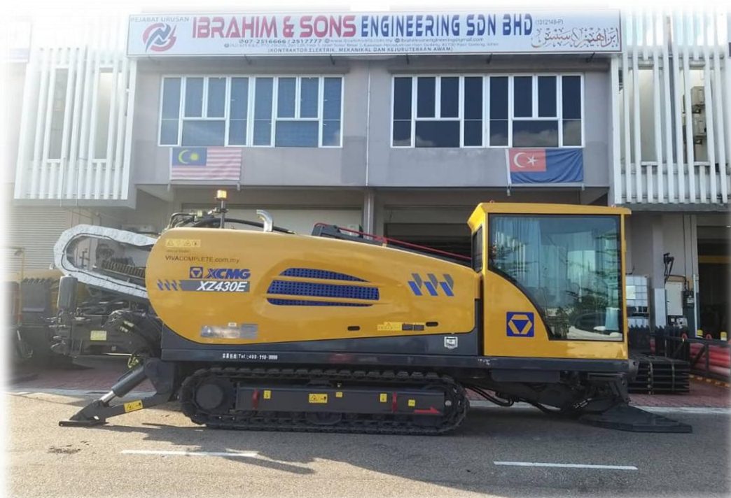
5 th HDD MACHINE 43 TONNE
